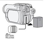
Before removing the battery, be sure to set the OFF/ ON switch to OFF and check that the status indicator is off before removing the battery.
